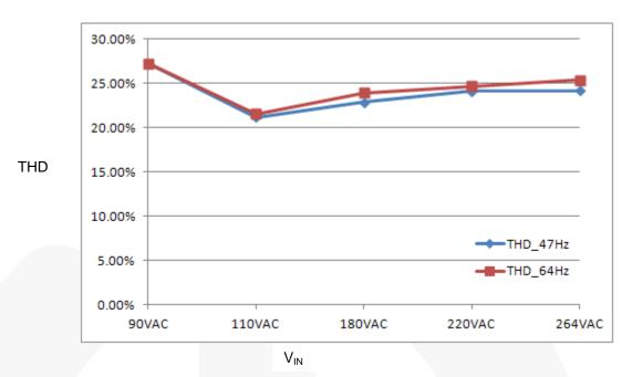
Figure 8. Total Harmonic Distortion
