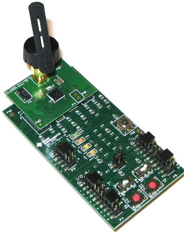
Figure 4 Sensor device using SmartRF05BB
