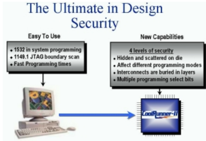
Figure 2.33 CoolRunner II Device Security
