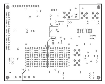
Figure 29. Board Layout, Layer 3
