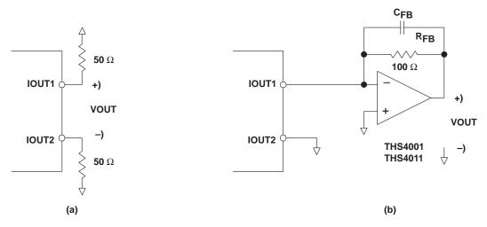
Figure 24. Differential and Single-Ended Output Configuration
