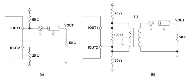
Figure 25. Driving a Doubly Terminated 50  $\Omega$  Cable
