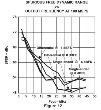
$\uparrow$  AV<sub>DD</sub> = DV<sub>DD</sub> = 5 V, IOUT<sub>FS</sub> = 20 mA, differential transformer coupled output, 50  $\Omega$  doubly terminated load, T<sub>A</sub> = 25°C (unless otherwise noted.)
