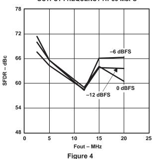
$\uparrow$  AV<sub>DD</sub> = DV<sub>DD</sub> = 5 V, IOUT<sub>FS</sub> = 20 mA, differential transformer coupled output, 50  $\Omega$  doubly terminated load, T<sub>A</sub> = 25°C (unless otherwise noted.)
