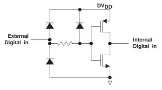
Figure 21. Digital Equivalent Input
