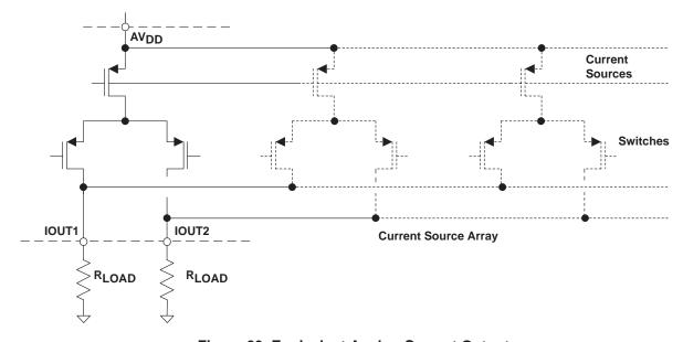
Figure 23. Equivalent Analog Current Output
