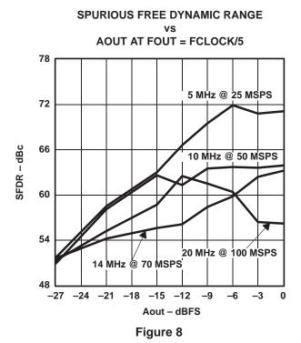
$^{\dagger}$  AV DD = DVDD = 5 V, IOUTFS = 20 mA, differential transformer coupled output, 50  $\Omega$  doubly terminated load, TA = 25°C (unless otherwise noted.)
