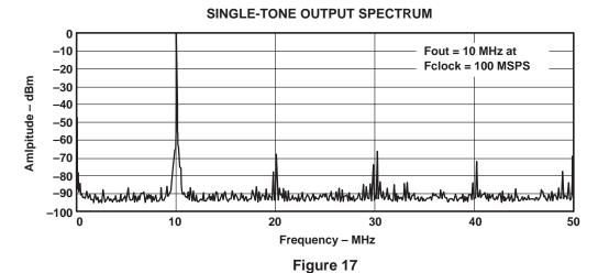
$\uparrow$  AV DD = DVDD = 5 V, IOUTFS = 20 mA, differential transformer coupled output, 50  $\Omega$  doubly terminated load, TA = 25°C (unless otherwise noted.)
