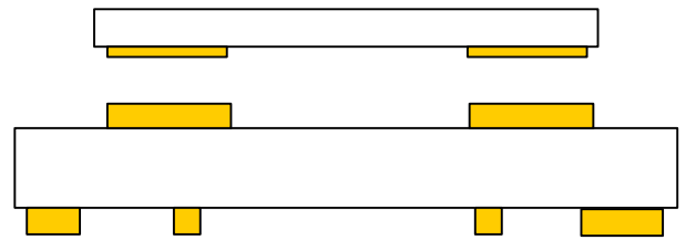
Figure 21. Correct PCB Top Metal Pattern Under Package
