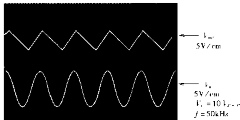
(b) A: \mu\text{A}741 SR = 0.3 \text{ V}/\mu\text{s}
